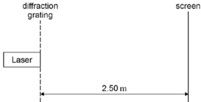
The laser has a wavelength of 628 nm. **Figure 2** shows part of the interference pattern that appears on the screen. A ruler gives the scale.
